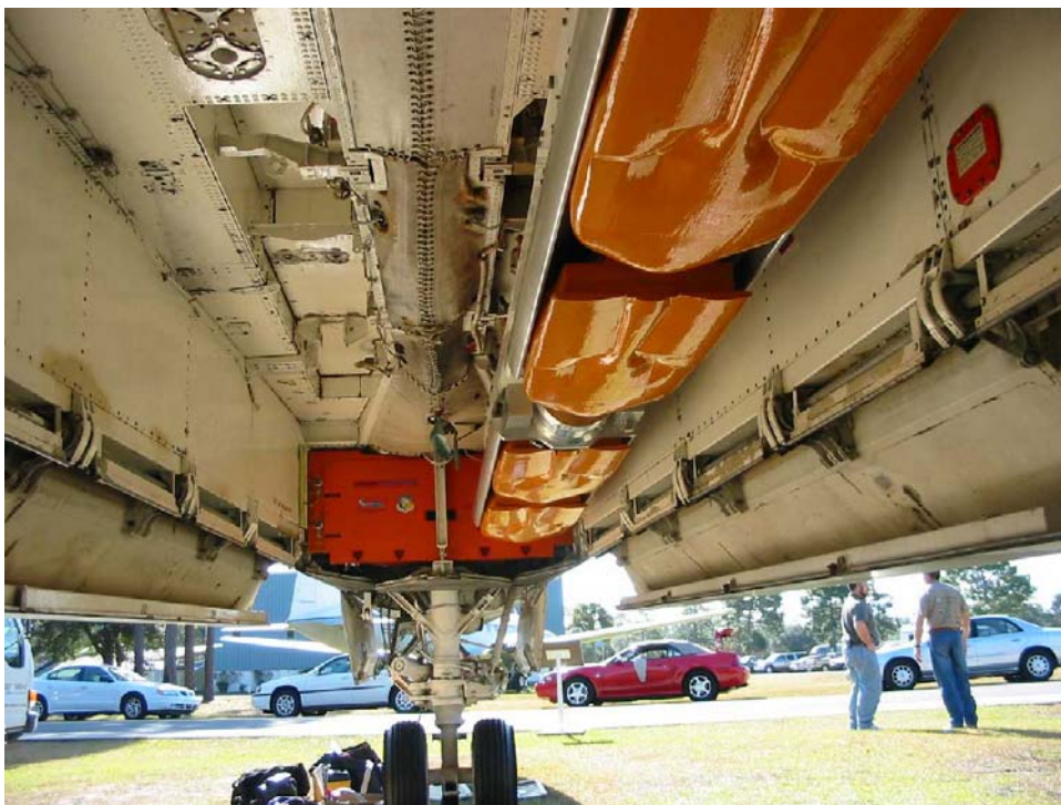
Figure 1. F-111E with the US AFRLs Powered LOW Cost Autonomous Attack System (PLOCAAS) Subpack during RAAF MIL-HDBK-1763 Fit Test at Eglin AFB.
